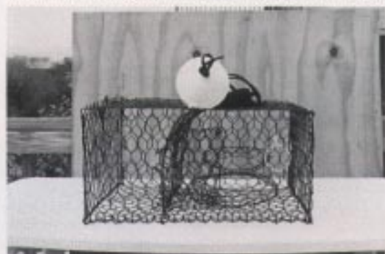
(6) Make hole in bottom for bait holder, and a door w/wire-loop hinges. Add tie-down strap, escape rings, and buoy.
