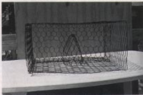
(3) Shape an 11"X14" piece into bait holder & attach. (Save scrap.) In center wall, cut and shape two entry slits to back.
